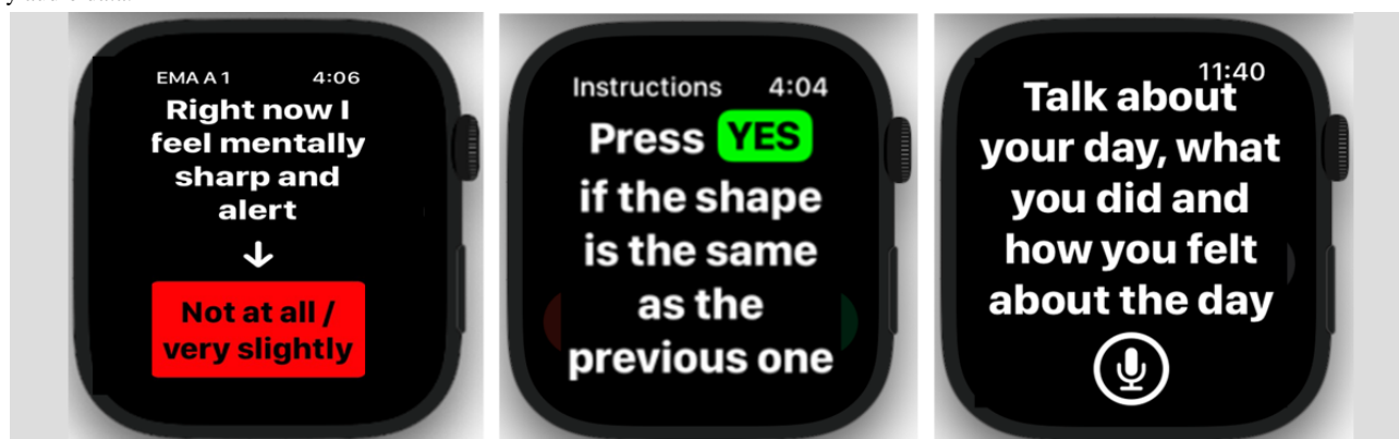
Figure 2. In addition to collecting sensor data, the smartwatch app queries the user for their current state, includes an n-back shape test, and collects daily audio data.
